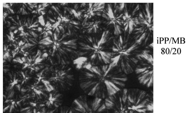
Fig. 2. Optical micrographs of isothermally crystallized ( T_c = 130^\circ\text{C} ) samples: (a) iPP; (b) iPP/MB 80:20 blend.
